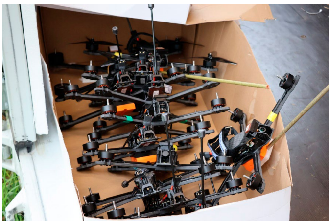
A box of interceptor drones equipped with 'aerial jousting sticks' used to hit the fixed-wing aircraft. Image: Oscar Warren/ASPI.
