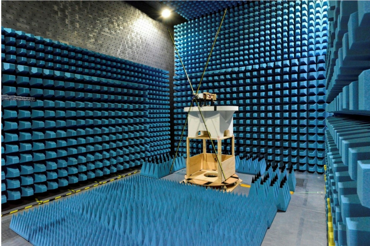
Image: Antenna characterisation testing of DSTG nanosatellite, Buccaneer Main Mission, with fully deployed high-frequency antenna in REDARC's anechoic chamber. Defence Images
